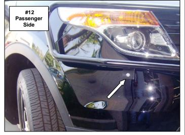
**Step-11** Align the push bumper and brush guard assembly with the vehicle and tighten all nuts and bolts. Remember to check and retighten the nuts and bolts periodically.
