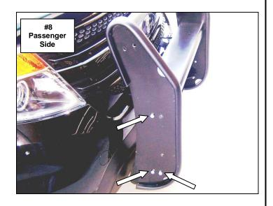
**Step-8** Attach the passenger side brush guard to the push bumper using (4) 3/8" x 1 1/4" hex bolts, (4) 3/8" lock washers and (4) 3/8" hex nuts. **Picture #9** Leave the nuts and bolts loose for final adjustment.
