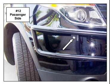
**Step-11** Align the push bumper and brush guard assembly with the vehicle and tighten all nuts and bolts. Remember to check and retighten the nuts and bolts periodically.
