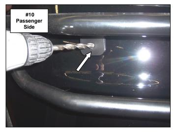
**Step-10** From behind the bumper fascia, position (1) 3/8" nut plate inside the channel of the brush guard bracket and secure the passenger side brush guard to the bumper fascia and brush guard bracket using the nut plate, (1) 3/8" x 1 1/4" hex bolt and (1) 3/8" lock washer. **Picture #11 & #12**
