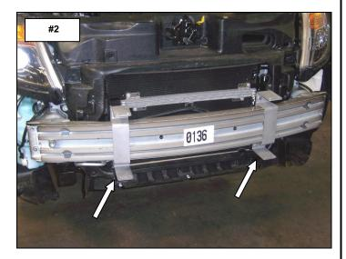
**Step-2** Beginning with the passenger side, remove the (2) 13mm head bolts securing the end of the steel impact beam to the frame. Install the passenger side brush guard bracket by positioning the bracket flanges inside the opening at the end of the impact beam, align the holes in the bracket with the threaded inserts in the frame and secure the bracket and impact beam to the frame using the factory bolts. **Picture #3**
