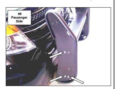
**Step-8** Attach the passenger side brush guard to the push bumper using (4) 3/8" x 1 1/4" hex bolts, (4) 3/8" lock washers and (4) 3/8" hex nuts. **Picture #9** Leave the nuts and bolts loose for final adjustment.
