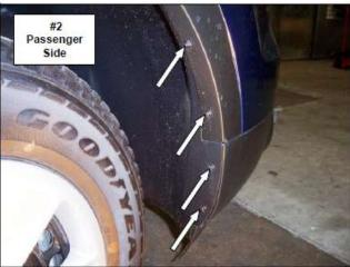
3. Remove the (9) hex bolts attaching the fascia to the core support and fender liner. Note: **Picture #4** shows the three Passenger side bolts and two center bolts only.
