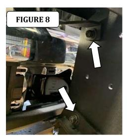
**Step-10** Align the Grille Guard with the front of the vehicle and tighten all bolts and nuts.
