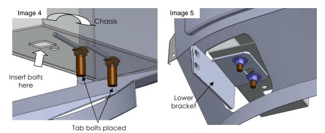
7. Place lower bracket on the bottom frame, fasten using 1/2" flat and lock washers and hex nuts. **Image 5**
