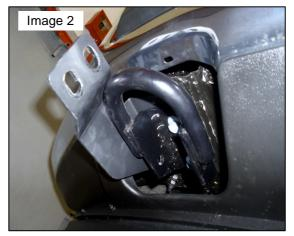
3. Slide lower bracket between the rear tow hook bolt and re-install the tow hook over the bracket. Re-attached using the factiry bolts removed in step 2. Image 2. Leave loose. Follow to step 8.
