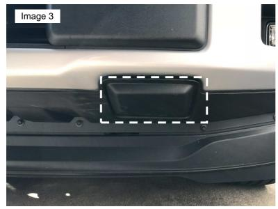
5. Align paper template to the edges shown at **Photo 3**, mark area to cut out and proceed. Repeat for opposite side, review simmetry.
