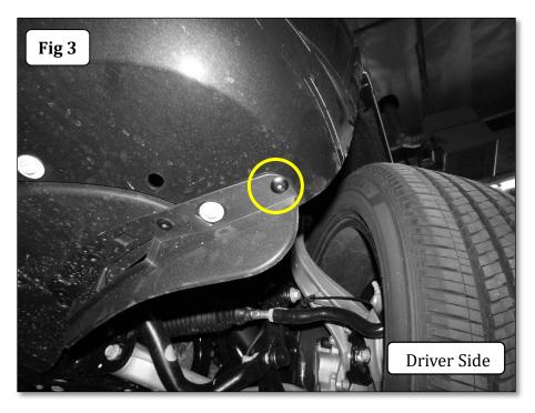
**Step-4** Using a 10mm socket remove the (10) screws attaching the lower fascia to engine splash shield, (Fig 4).
