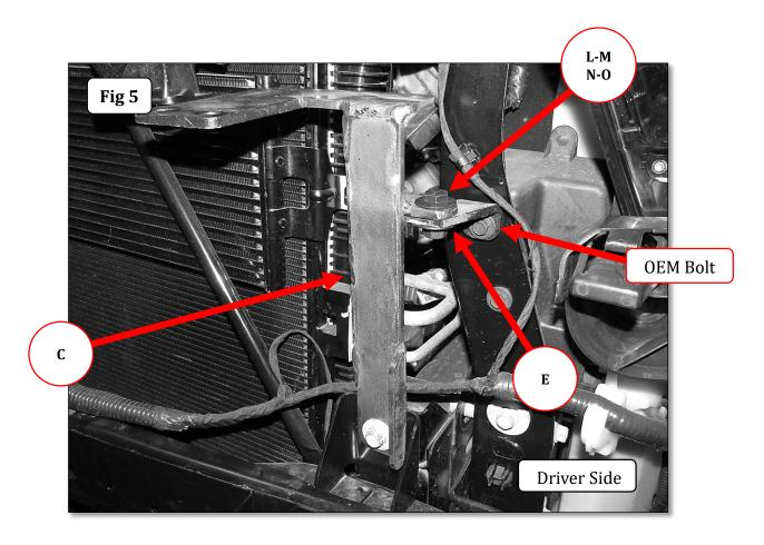
**Step-6** Reinstall the upper and lower fascia assembly.
