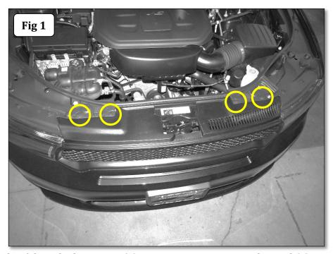
**Step-2** On each side of the vehicle remove (1) screw using an 8mm socket and (1) screw using a 10mm socket. Use diagonal-cutting pliers to remove (2) plastic rivets attaching the fender liner to the bumper cover, (Fig 2). **Note:** The OEM plastic rivets attaching the fender liner to the bumper cover will be replaced with the supplied Push-In Ribbed Shank Rivets.
