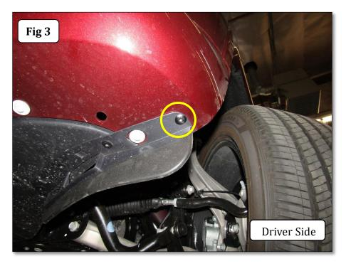
**Step-4** Using a 10mm socket remove the (13) screws attaching the bumper cover to engine splash shield, (Fig 4).
