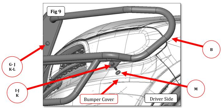
**Step-12** Attach the three remaining holes in the brush guard to the push bumper using (2) 3/8" x 1" hex bolts, (1) 3/8" x 1  $\frac{1}{4}$ " Hex Bolt, (3) 3/8" flat washers, (3) 3/8" lock washers and (3) 3/8" hex nuts, (Fig 10). Leave the nuts and bolts loose for final adjustment.
