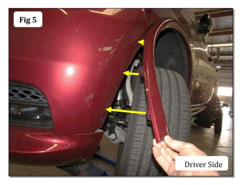
**Step-6** Pull out on the corners of the bumper cover to release it from the locking strip located on each side and under each headlight, (Fig 6). Note: On the passenger side disconnect the fog light wiring harness from the vehicle harness if the vehicle is so equipped. Remove the bumper cover from the vehicle.
