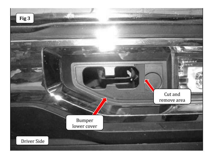
**Step-4** From the opening at the end of the driver side frame, position (1) M12 t-bolt inside the frame with the bolt extending out through the obround shape hole on the side of the frame. Install (1) vinyl gasket on the bolt to keep the t-bolt from falling back into the frame. Note: To ease installation use the supplied pull wire to fish the t-bolt from the opening and out through hole in the frame.
