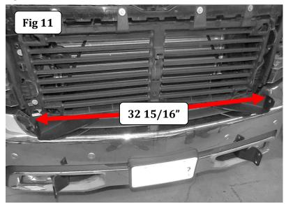
**Step-13** With assistance, hold the push bumer up in position on the outside of the upper and lower mounting brackets.
