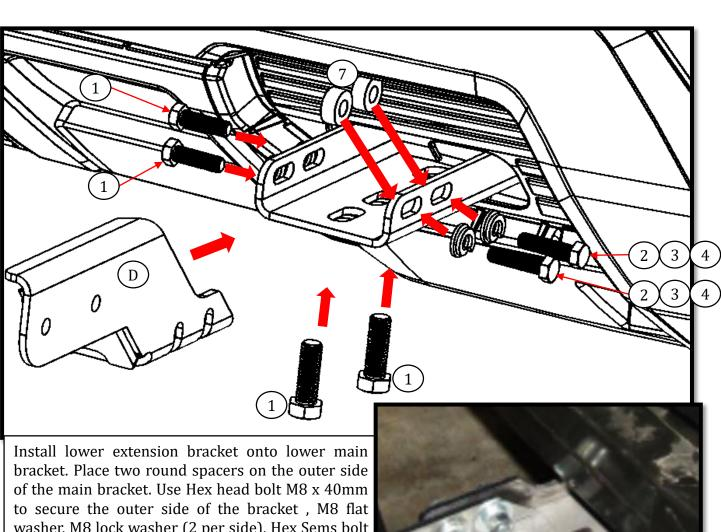
washer, M8 lock washer (2 per side), Hex Sems bolt  $M8 \times 30 mm$  to secure the inner side of the frame bracket. The bottom side can be secured using Hex Sems bolt M8 x 30mm (2 per side). Repeat process for both sides.
