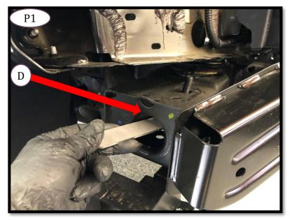
**Step-2** With the bumper cover removed, locate the large circular opening. Introduce the bolt plate with the threads exposed as a stud. Picture (1) is referencing the passenger side.
