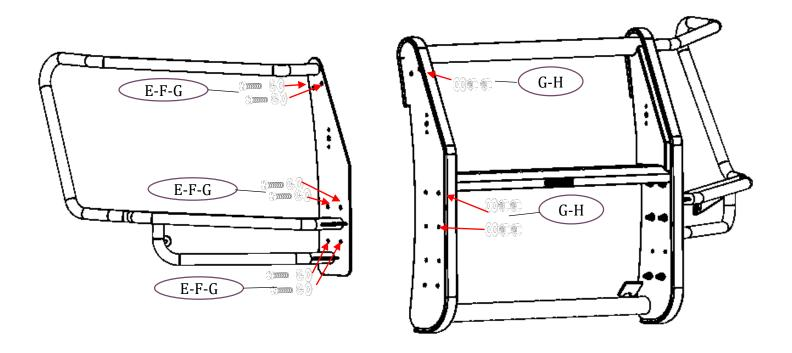
**Step -5** Install headlight wraps onto center grill guard. Use  $3/8" \times 1 \%"$  hex bolt (6 per side), 3/8" lock washer (6 per side), 3/8" flat washer (12 per side) and 3/8" hex nut (6 per side). Leave finger tight and adjust to fit to your satisfaction. Repeat step for both sides, if the bumper was already installed, replace the auxiliary bracket bolts with the above mentioned.
