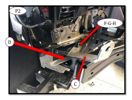
**Step-3** With the bolt plate positioned correctly, install the mounting bracket and secure it using 3/8" flat washer, 3/8" lock washer, 3/8" hex nut. Leave finger tight as you will be fastening it at a later step (picture 2). Repeat process on driver side.
