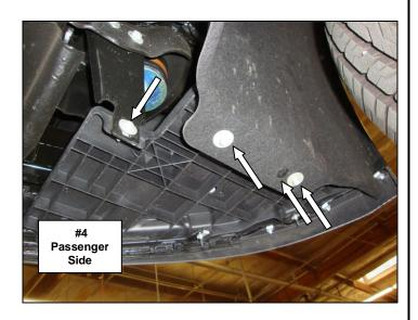
Step-5 On each side, remove (1) 7mm (head) screw securing the fascia to the bumper impact beam bracket, (Photo 5).
