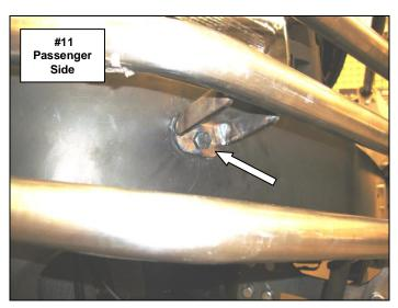
**Step-14** Align the push bumper and brush guard assembly with the vehicle and tighten all factory and supplied nuts and bolts securing the push bumper and brush guard assembly and brackets.
