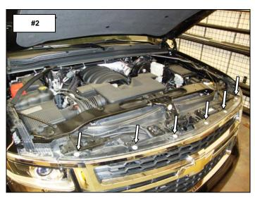
Step-3 On each side, remove the (6) 7mm head screws securing the fender liner to the fascia, (Photo 3).
