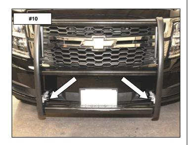
Step-11 Align the push bumper with the vehicle and tighten all factory and supplied nuts and bolts, (Photo 11).
