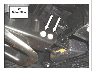
**Step-2** From the opening at the end of the frame, place one of the 5/16" bolt plates inside the frame, and position the bolt plate so the threads extend out through the hole in the bottom of the frame, **(Photo 3).**
