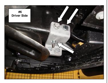
**Step-6** Align the holes and attach the auxiliary bracket to the driver side main bracket using (2) M12 x 40mm hex bolts, (2) M12 flat washers, (2) M12 Lock washers and (2) M12 hex nuts. Leave the nuts and bolts loose for final adjustment, **(Photo 7 & 8).**
