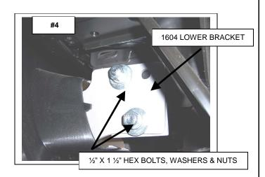
**STEP 7:** ATTACH THE GRILLE GUARD ASSEMBLY TO THE OUTSIDE OF THE LOWER MOUNTING BRACKETS USING (4) 1/2" X 1 1/2" HEX BOLTS, (8) FLAT WASHERS, (4) LOCK WASHERS AND (4) HEX NUTS. DO NOT TIGHTEN. **PHOTO #5**
