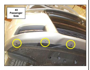
Step-3 Remove the (3) screws securing the brake cooling duct to the fender well, (Photo 3).
