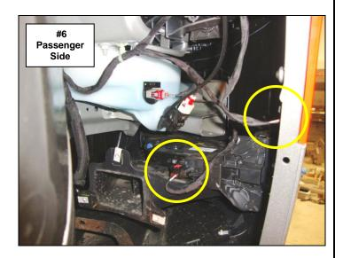
**Step-6** With assistance pull out on the sides of the fascia and forward to remove it from the vehicle.
