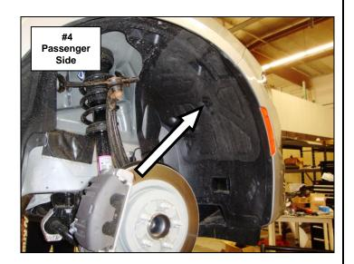
**Step-5** Pull back the front section of the fender well and remove the (2) bolts securing the bumper fascia to the fender. Disconnect (unplug) the side marker light wiring and If equipped disconnect the fog light, (Photo 5 & 6). Repeat steps 3, 4 and 5 on the driver side of the vehicle.
