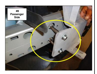
**Step-9** Attach the bracket to the impact beam. Position the flange of the bracket approximately 11 1/2" from the end of the impact beam and tighten the bolts, (Photo 9 &10). Repeat steps 8 and 9 for the driver side bracket.
