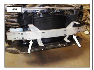
**Step-10** The bumper insulator must be notched (top and bottom) to properly fit around the brackets, (Photo 11 &12). Remove the insulator from the bumper fascia. Position the insulator up to the bumper and mark the bracket locations. Notch the insulator and check fit by returning the insulator to the bumper until the proper fit is achieved. Re-install the bumper insulator in the bumper fascia.
