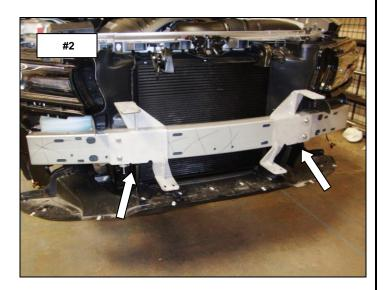
**Step-2** Beginning with the passenger side locate the holes, top and bottom at the end of the bumper impact beam, (Photo 3).
