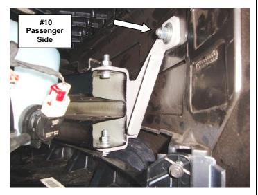
**Step-10** Align the push bumper and brush guard assembly and tighten all nuts and bolts securing the push bumper, brush guard assembly and brackets, (Photo 11).
