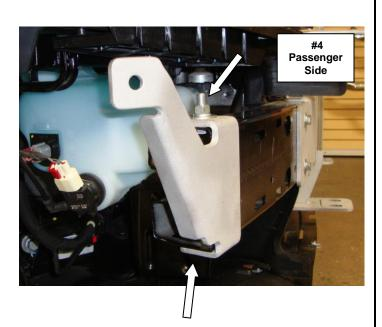
**Step-4** The ends of the bumper insulator must be notched to properly fit around the brackets, (Photo 5). Position the insulator up to the bumper and mark the bracket locations.
