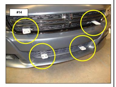
**Step-13** Attach the push bumper to the brackets using the supplied 3/8" x 1 1/4" hex bolts, 3/8" flat washers, 3/8" lock washers and 3/8" hex nuts, (Photo 15).
