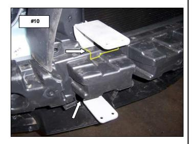
Step-12 An area in each side of the upper and lower grille must be cut out for the brackets to extend through.
