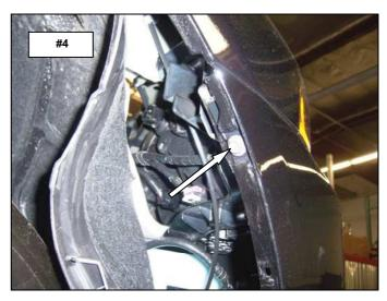
**Step-5** With assistance pull out on the sides to unsnap the corners of the fascia and forward to remove it from the vehicle.
