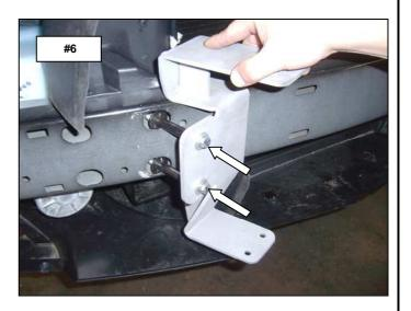
**Step-8** Position the flange of the bracket approximately 12" from the end of the bumper and attach the bracket to the bumper. **Picture #7**
