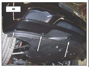
Step-3 Remove the plastic rivets (3 per side) securing the fender well to the bumper fascia. Picture #3
