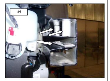
**Step-4** Align the spacers and nut plate assembly with the holes in the bumper. Position the passenger side brush guard bracket on top of the bumper and secure the bracket to the bumper using the 3/8" x 3 1/2" hex bolts, lock washers, flat washers and u-nut plate. Leave the bolts loose for final adjustment. **Picture #5** Repeat the above steps to install the driver side brush guard bracket.
