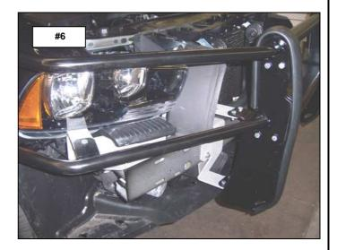
**Step-6** Remove the push bumper and brush guards assembled from the brackets. Do not loosen or remove the bolts attaching the brackets to the bumper.
