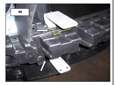
**Step-8** Attach the push bumper and brush guard assembly to the brackets using the 3/8" hex bolts, flat washers, lock washers and hex nuts. Tighten all nuts and bolts.
