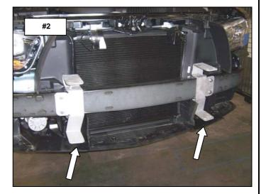
**Step-2** Beginning with the passenger side locate the holes in the top and channel section of the steel bumper. **Picture #3**
