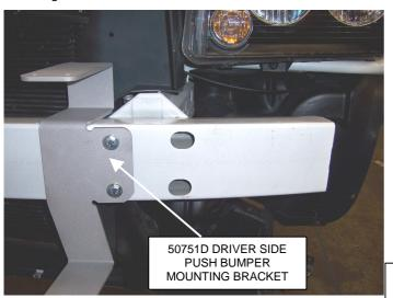
**STEP 2.** Assemble and attach the driver side brush guard bracket to the bumper using one of the 50755 clamp brackets, 3/8" x 1" hex bolts, washers and nuts as shown. Do not tighten. Repeat this step for the passenger side.
