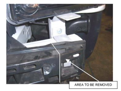
**STEP 8.** Reinstall the bumper fascia. Attach the push bumper and brush guard assembly to the mounting brackets using the 3/8" x 1" hex bolts, flat washers, lock washers and hex nuts. Tighten all mounting nuts and bolts.
