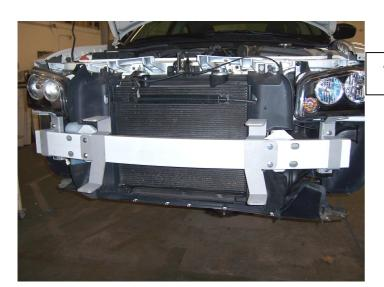
**STEP 6.** The bumper insulator must be notched **(top and bottom)** and the ends must be trimmed to properly fit around the push bumper and brush guard mounting brackets. Unsnap the bumper insulator from the bumper fascia. Position the insulator up to the bumper and mark the bracket locations.
