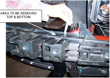
**STEP 7.** Notch and trim the bumper insulator. Check the fit by returning the insulator to the bumper. Once the proper fit is achieved. Reattach the insulator to the bumper fascia.
