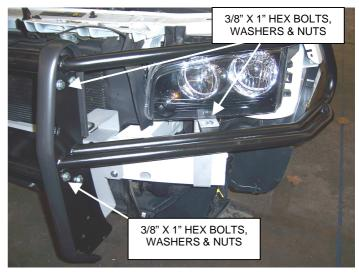
**STEP 5.** Remove the push bumper and brush guard assembly from the mounting brackets. Do not loosen or remove the brackets.
