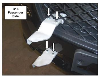
**Step-9** Attach the push bumper to each of the extension brackets using (2) 3/8" x 1" hex bolts, (2) 3/8" lock washers and (2) 3/8" hex nuts. Leave the nuts and bolts loose for final adjustment. **Picture #17 & #18**
