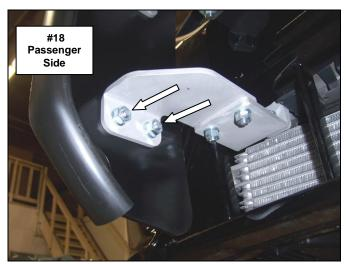
Step-10 Align the push bumper with the vehicle and tighten all nuts and bolts. Picture #19 & #20
