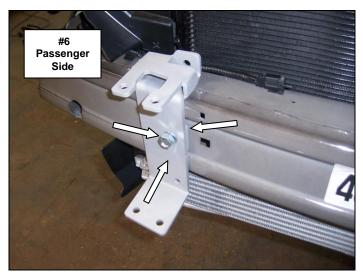
**Step-3** Insert the top of the passenger side clamp bracket through the gap between the impact beam and auxiliary cooler, and then rotate the bracket into position. Slide the bracket to the left and align the holes in the clamp bracket with the main bracket. Secure the clamp bracket to the main bracket using (2) 3/8" x 1" carriage bolts, (2) 3/8" lock washers and (2) 3/8" hex nuts. **Picture #7 & #8** Leave the nuts and bolts loose for final adjustment.
