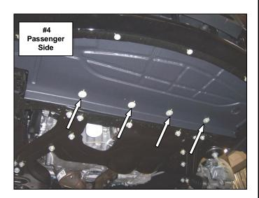
**Step-5** With assistance pull out on the sides to release the corners of the bumper fascia and forward to remove it from the vehicle.
