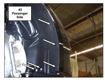
**Step-3** Pull back the fender liner and remove the Phillips screw and plastic fastener attaching the fascia to the fender. **Picture #3**
