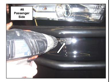
**Step-8** From Behind the bumper fascia, Position (1) 3/8" nut plate inside the channel of the brush guard bracket and secure the passenger side brush guard to the bumper fascia and bracket using the nut plate, (1) 3/8" x 1 1/4" hex bolt and (1) 3/8" lock washer. **Picture #9 & #10**
