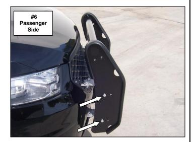
**Step-6** Attach the passenger side brush guard to the push bumper using (4) 3/8" x 1 1/4" hex bolts, (4) 3/8" lock washers and (4) 3/8" hex nuts. **Picture #7** Leave the nuts and bolts loose for final adjustment.
