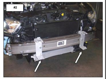
**Step-2** Beginning with the passenger side, remove the (2) 13mm head bolts securing the end of the steel impact beam to the frame. **Picture #3**
