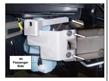
**Step-4** Refer to the installation instructions included with the push bumper (#5039) to notch the bumper insulator and complete the push bumper bracket installation. **Picture #5**
