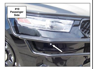
**Step-9** Align the push bumper and brush guard assembly with the vehicle and tighten all nuts and bolts. Remember to check and retighten the nuts and bolts periodically.
