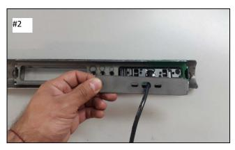
**Step-3** Place one spacer plate over the light bracket and attach the light using the screws M3.5x10 (included with the light). **See figure 5.**
