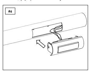
**Step-7** Secure the light bar assembly to the light bar tube using two 1/4"x 3/4" allen head bolt and lock washers. **See image 6 & 7.**
