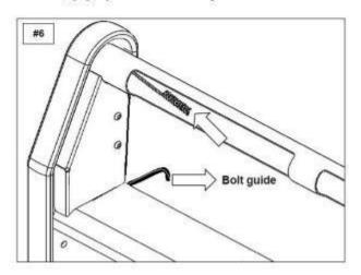
**Step-8** Secure the light bar assembly to the light bar tube using two 1/4"x 1 3/4" allen head bolt. **See figure 8**.
