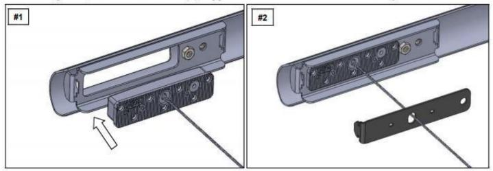
Step-3 Attach the light using the screws #4-40 x 1/4". See figure 5.
