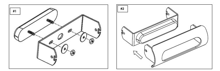
**Step-3** Assemble the light mounting bracket and attach all together using (1) #6 x 3/4" button allen bolt, (1) #6 flat washer and (1) #6 hex lock nut per side. **Image 3 & 4**.
