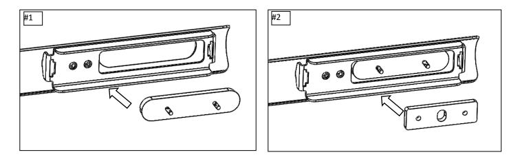
**Step-3** Place the light bracket on top of the light, then push the light bracket to the left. Place (1) support bracket and secure the assembly using (1) 1/4" lock washer and (1) 1/4" x 1/2" allen head bolt. **See figure 2, 3 & 4. NOTE:** Place (1) support bracket to each extreme of the lighted bar.
