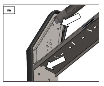
**Step-9** Secure the light bar assembly to the light bar tube using two 1/4"x 1 <sup>3</sup>/<sub>4</sub>" allen head bolt. **See figure 8.**
