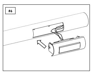
**Step-8** Secure the light bar assembly to the light bar tube using two 1/4"x 3/4" allen head bolt and lock washers. **See image 6 & 7.**
