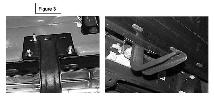
**3.** Locate the (3) threaded studs on the inner rocker panel at the center and rear of the cab and repeat step 2 to install two of the brackets using the supplied hardware. Note: The front mounting location is shown in Figure 3. The center and rear mounting locations are similar.
