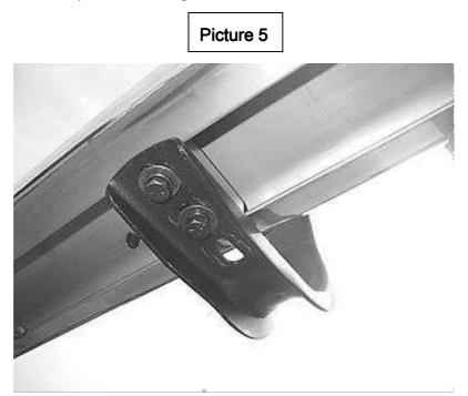
**6.** Repeat steps to install the passenger side brackets and side step. Remember to check and retighten the nuts and bolts every six months.
