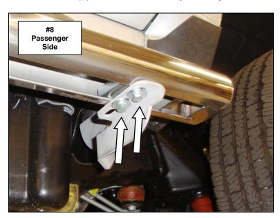
Step- 7 Align the side bar with the vehicle and tighten all side bar and bracket nuts and bolts.
