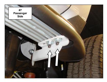
If installing **4**", **5**" or **6**" Channel Mount side bars attach the side bar to each bracket using (1) U-bracket (2) 5/16" hex bolts (2) 5/16" lock washers and (2) 5/16" flat washers, (Photo 8).
