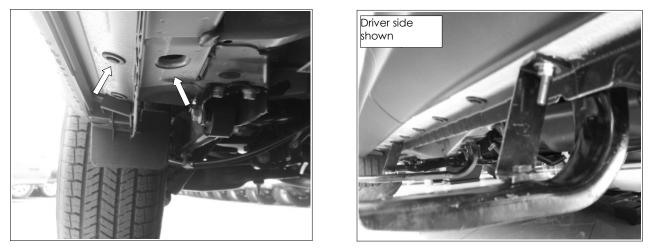
12. To install the rear bracket, locate the existing obround in the rear of the rocker panel (see picture 7) and insert a 1/2" bolt plate. Attach the rear bracket to the 1/2" bolt plate using (1) flat washer, (1) lock washer and (1) hex nut 1/2". Attach the other end of the auxiliary rear bracket to the rear bracket with (1) hex bolt  $5/16 \times 1$ ", (1) flat washer, (1) lock washer and (1) hex nut 5/16". (See picture 8). Do not tighten. Repeat this procedure to install the passenger side.
