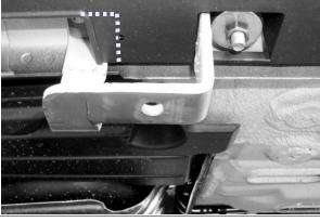
8. Locate the existing hole behind the auxiliary rear bracket. Insert a 3/8" bolt plate then place the rear bracket and secure using (1) 3/8" flat and lock washers and (1) 3/8" hex nut. Picture 7.
