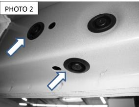
**5. 2** Install M8 Clip-Nuts in the rocker panel with the threaded end centered over the smaller hole, (**PHOTO 3**).
