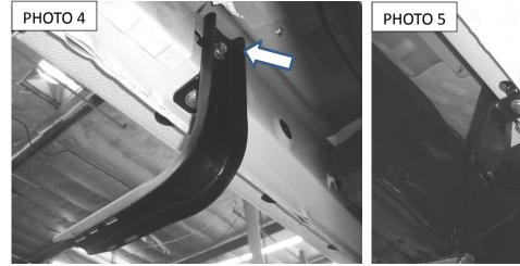
**7.** Locate the plastic plugs and holes in the rocker panel and repeat steps1-3 to install the two center and one rear bracket.
