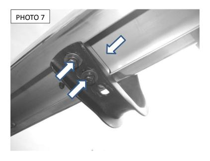
10. If installing 415 side steps place the side step on top of the mounting brackets, align the threaded holes in the side step with the holes in the mounting brackets and secure the side step to each bracket using (2) 5/16" x 1" hex bolts, (2) 5/16" lock washers and (2) 5/16" flat washers. Align the side step with the vehicle then tighten all side step and mounting bracket nuts and bolts, and factory body bolt. (PHOTO 8)
