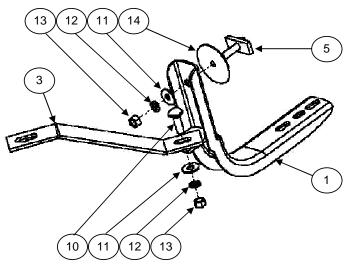
Use ratchet & 19mm - 9/16" hex socket. Remove the bolt OEM with: ratchet & 19mm hex socket.
