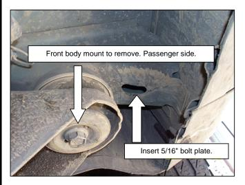
3. Install the front bracket and attach with bolts before removed. Locates the hole that is in the rocker of the vehicle and inserts 5/16" bolt plate.
