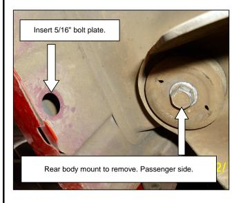
7. Install the middle bracket and attach with bolts before removed. Locates to the rubber plug that is in the rocker of the vehicle, remove and insert 5/16" bolt plate.
