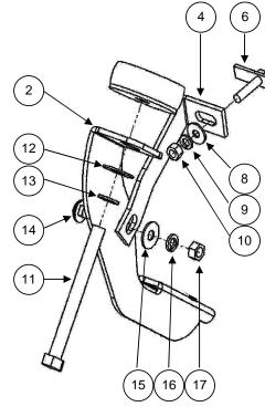
Use ratchet & 18mm - 19mm - 9/16" - 1/2" hex socket. Remove the bolt OEM with: ratchet & 18mm hex socket.
