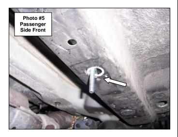
**Step-4** Attach the passenger side front bracket to the bottom of the frame using the 5/16" x 1 ½" t-bolt, (1) 5/16" flat washer, (1) 5/16" lock washer and (1) 5/16" hex nut, (**Photo #6**). Leave the hex nut loose for final adjustment.
