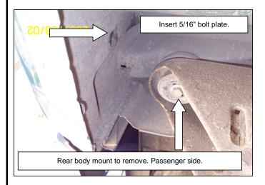
7. Install the middle bracket and attach with bolts before removed. Locates to the rubber plug that is in the rocker pannel of the vehicle, remove and insert 5/16" bolt plate.
