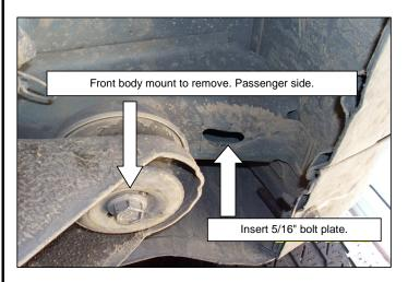
**3.** Install the front bracket and attach with bolts before removed. Locates the hole that is in the rocker pannel of the vehicle and inserts 5/16" bolt plate. Mounts the front auxiliary bracket and attach with: 5/16" flat and lock washers, 5/16" hex nut. In the other side of the bracket attach with the front bracket: 3/8 x 1" carriage head bolt, 3/8" flat and lock washers, 3/8" hex nut. **SEE PICTURE 1, ILLUSTRATION 3.** Leave loose.
