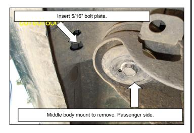
**5.** Install the middle bracket and attach with bolts before removed. Locates the hole that is in the rocker pannel of the vehicle and inserts 5/16" bolt plate. Mounts the middle auxiliary bracket and attach with: 5/16" flat and lock washers, 5/16" hex nut. In the other side of the bracket attach with the middle bracket: 3/8 x 1" carriage head bolt, 3/8" flat and lock washers, 3/8" hex nut. **SEE PICTURE 2, ILLUSTRATION 4.** Leave loose.
