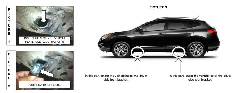
5.- Place the driver side front bracket and secure with: 3/8" flat and lock washer, 3/8" hex nut. Leave loose. SEE ILLUSTRATION 1.
