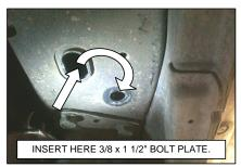
8.- In the larger hole also insert 3/8 x 1 1/2" bolt plate, but without using 3/8" bolt guide, Make sure they are as  $\ensuremath{\text{PICTURE 6.}}$
