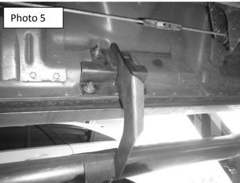
4. Locate the three M8 welded bolts in the rocker panel near the end of the cab. Install the rear bracket using (3) 5/16" flat washers Gray P., (3) 5/16" spring lock washers Gray P. and (3) M8 hex nut Gray P. Leave the nuts loose for final adjustment. (Photo 6 & 7)
