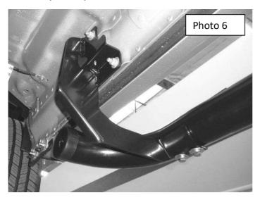
6. Align the side step with the vehicle and tighten all bracket and side step nuts and bolts. Repeat the above steps to install the driver side brackets and side step. Remember to check and retighten the nuts and bolts every six months.
