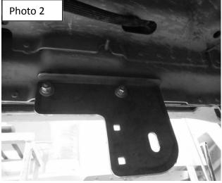
2. Install the auxiliary bracket using (1) b M8 hex nut Gray P., (1) 5/16" flat washer Gray P. and (1) 5/16" spring lock washer Gray P. Then attach the auxiliary bracket to the front bracket using (2) 5/16" carriage head bolt Black P., (2) 5/16" flat washers Black P., (2) 5/16"spring lock washers Black P. and (2) 5/16" hex nuts Black P. Leave loose for final adjustment. (Photo 3)
