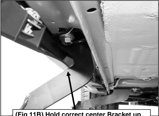
(Fig 11B) Hold correct center Bracket up in place to determine area to cut from bottom edge of rocker panel cover
