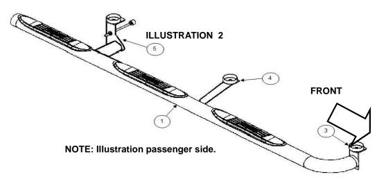
4. Side bar set consists of a driver and passenger side. Make sure to determinate the correct side before installation. See illustration 1.
