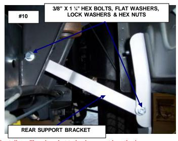
(For 2013 and newer models, drilling might be required to install auxiliary bracket to body mount location)
