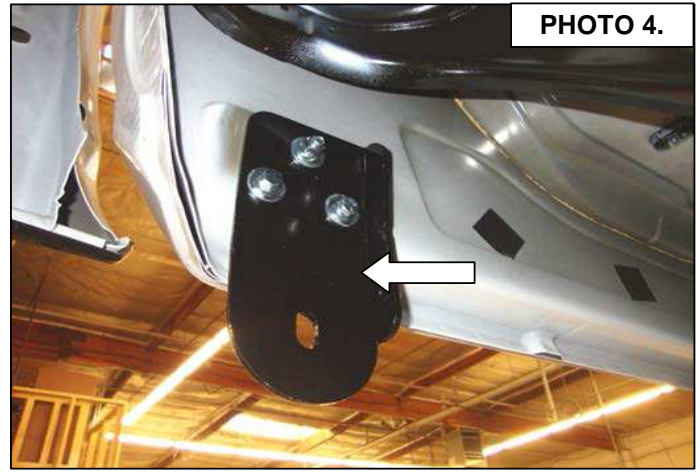
The rear bracket installed, photo driver's side rear shown.
