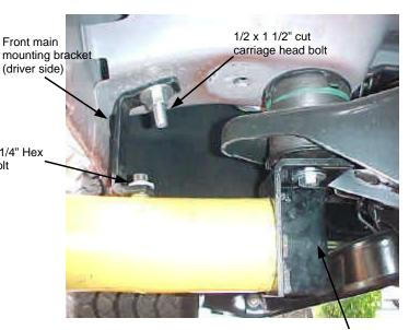
Front auxiliary mounting bracket (driver side)
