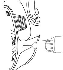
Once Hole is drilled and switch wires are pulled into vehicle crimp supplied connectors onto the 3 wires.
