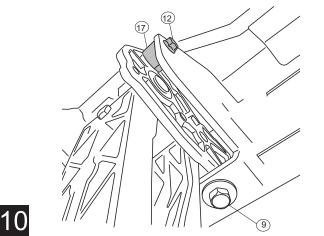
Using a 13mm socket Torque linkage bolts 4x (9) from step 3 to 16 ft-lbs. Next use a 10mm socket, torque linkage spacer bolt 2x (13) from step 6 to 8 ft-lbs. Once linkages are tight cycle board to verify steps deploy under own weight.
