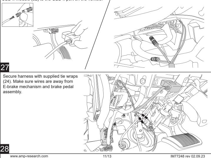
**OBD II install:** Use Supplied Posi-Lock connectors to attach the Plug and Play Module to the Harness. Attach matching colors on the harness to the wires on the module. Plug in module to OBD II port on the vehicle. Secure harness with supplied tie wraps.
