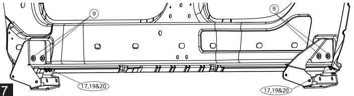
Insert and position 6 Carriage bolts (16) into slot on rail (4). Insert from either end of rail. Using Flange Nuts (10) provided assemble rail to Brackets using the 2 outer bolts on each side. Next install Flange Bolt (14) and Flange Nut (10) onto bracket tab. *Torque flange nuts to 16ft-Ibs.* Next install Light Bracket (29) using Flange Nut (10), leave loose to allow for adjustment. Driver side shown. Dimensions shown are for reference.
