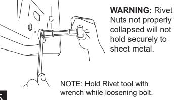
Once rivet nuts are in place use a screwdriver to push back tab in hole to avoid interference with linkage mount.
