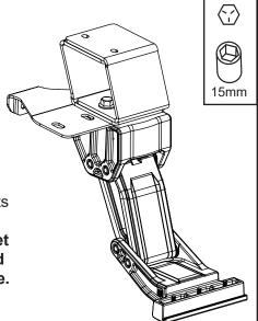
Using a 13mm socket assemble frame mount onto lateral mount using bolts (#10) and Captive washer nuts (#13). Torque to 16ft-lbs.
